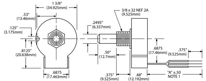
1. "A" Cable length standard 7 1/2 in. (190.5mm)
